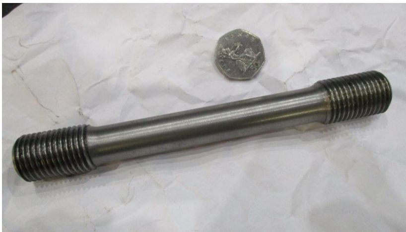
Sample of a new steel stay, each one measured and machined to fit
