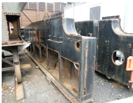
OLD TANKS BEING STRIPPED DOWN FOR USABLE FITTINGS & PATTERNS
