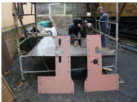
RUNNING PLATES FOR BOTH SIDES OF THE FOOTPLATE AREA NOTE CUT-OUTS FOR THE HANDBRAKE AND, REVERSING & SANDING LEVERS. IN THE BACKGROUND PHIL AND TERRY DRILLING THE NEW BUNKER FLOOR
