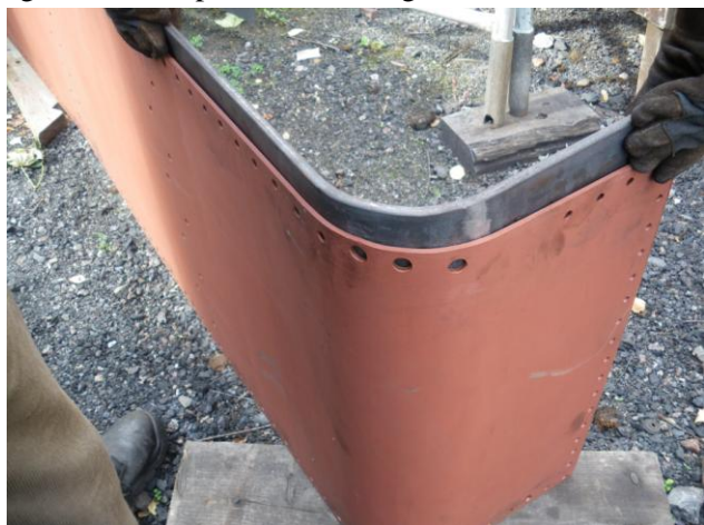
Checking the radius of the butt strip linking upper and lower rear sheets.
