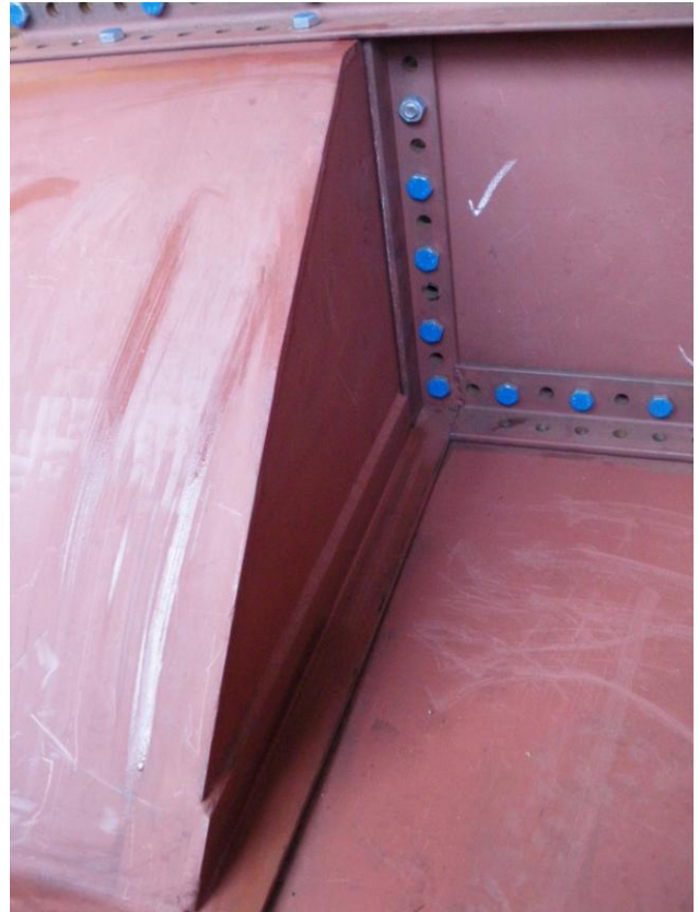
The welded 'box' seen in part on the left covers the sloping section of the loco mainframes, where they drop from footplate level to bunker base level.
