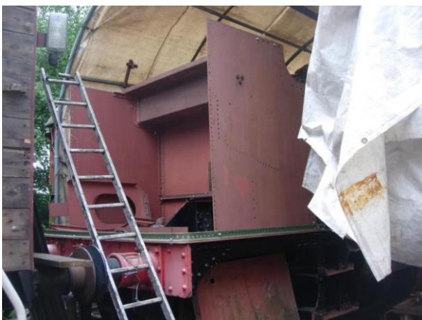
The bunker taking shape and a trial fitting of the baffles
